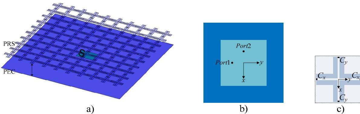
Fig. 1. PRS antenna with independent beamwidth control: a) the assembled antenna; b) the source; c) the cell.
