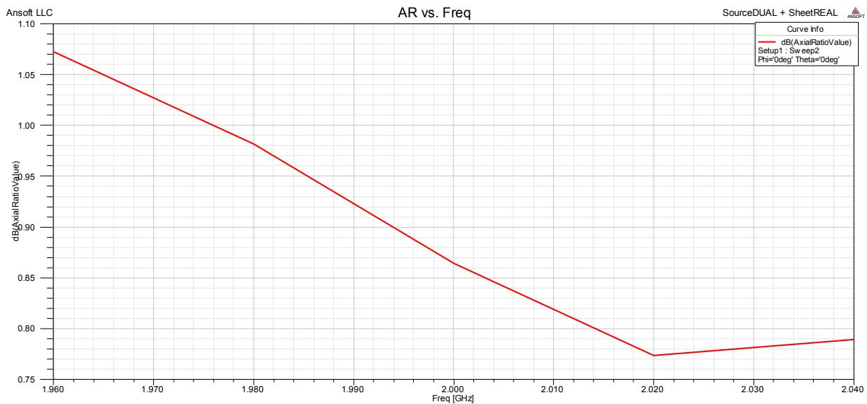
Fig. 4. Axial ratio in normal direction.
