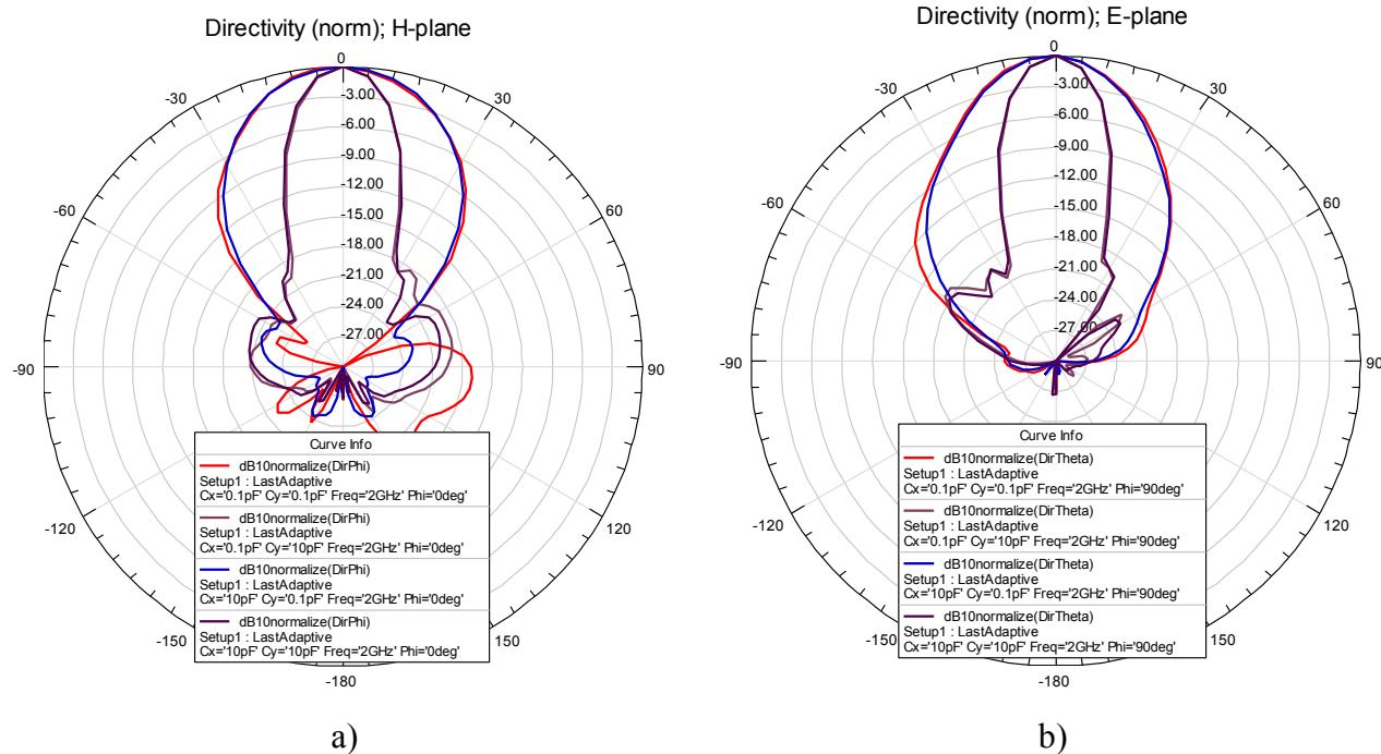
Fig. 3. Normalized directivity of the PRS antenna with independent beamwidth control (Port1 excited): a) H-plane; b) E-plane.
