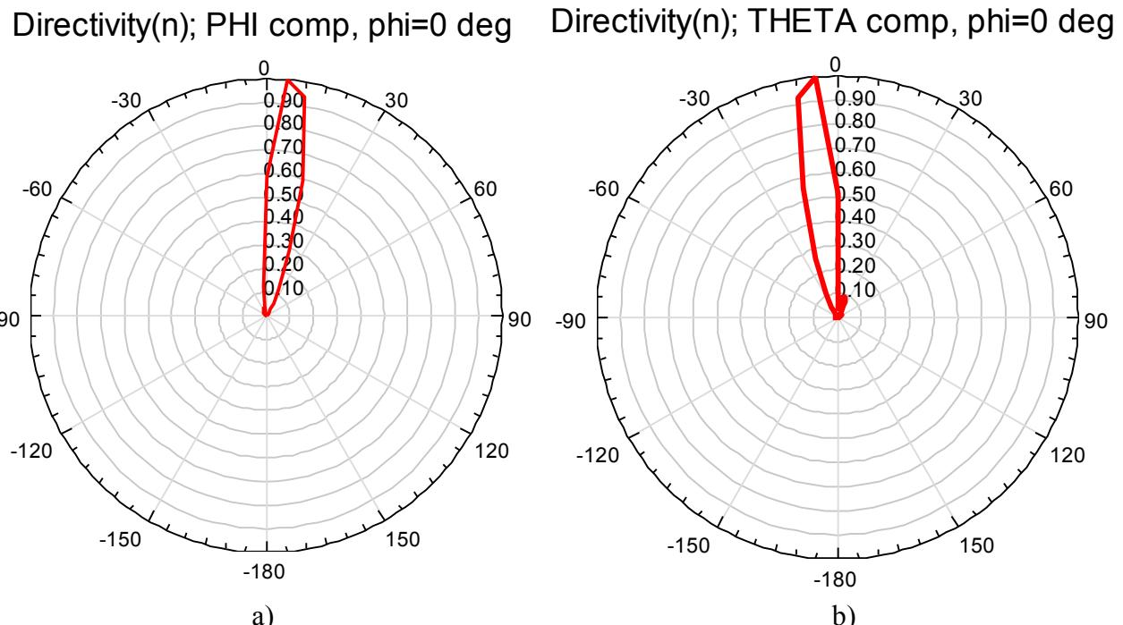
Fig. 5. Normalized directivity of the PRS antenna with phased array as a source: a)  $x$ -polarization; b)  $y$ -polarization.
