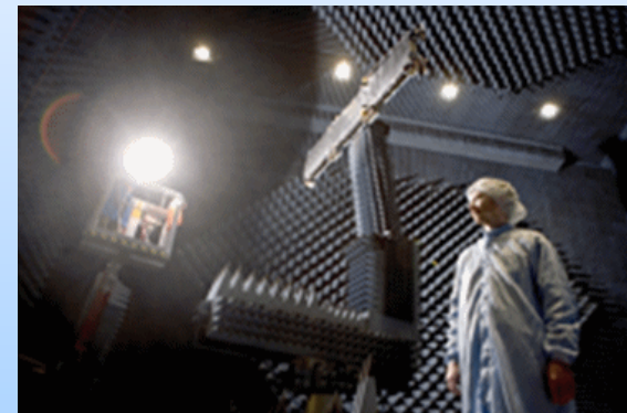
Measurement of radiometer antenna system for ESA's Soil Moisture and Ocean Salinity mission at the DTU-ESA Spherical Near- Field Antenna Test Facility
