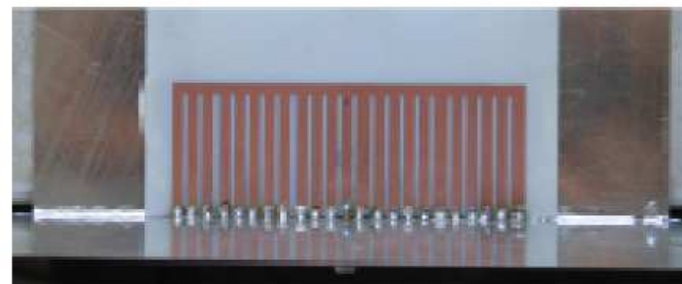
Folded monopole 2.4 GHz antenna closely spaced over PEC thickness d/\lambda \sim 0.01 (CTU)
