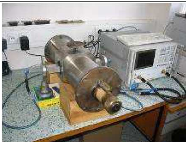
Fabry-Perot resonator with lens antennas model and testing (CTU)
